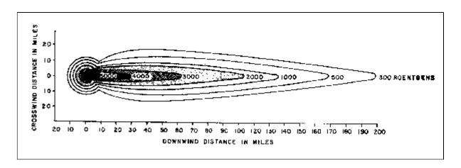
This was the fallout pattern 36 hours after a single 15-megaton thermonuclear device (the Bravo shot of Operation Castle at Bikini Atoll - March 1, 1954) was detonated. The eventual extension of the fallout was more than 20 miles upwind and over 320 miles downwind. The width in cross section was variable, the maximum being over 60 miles. This means there was substantial fallout contamination over an area of more than 7000 square miles.
